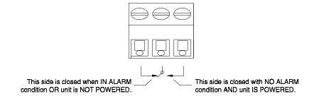
Figure 3-2: Contact ID for FAILSAFE Relay Operation
